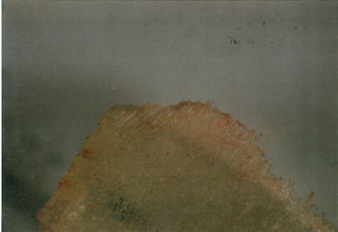
Figure 4 Optical micrographs of VGR I exposed to phenol red solution at room temperature for 40 min, X68.
